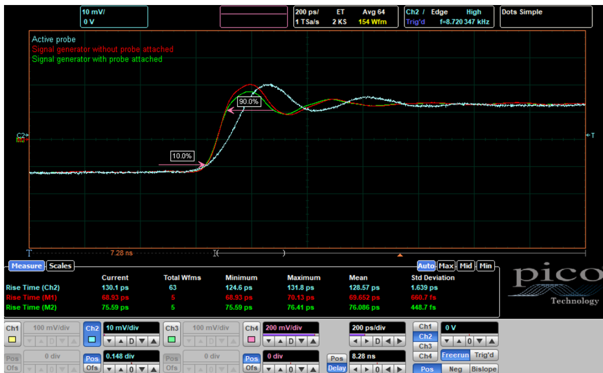
Figure 4. Rise time measurement using fast edge (70 ps) from fast signal generator. Blue line is output from probe, sensing signal via exposed coplanar waveguide. Red line is signal generator signal measured directly by oscilloscope without probe attached. Green line is signal generator signal measured directly by oscilloscope with probe attached. Probe rise time of around 130 ps is measured. Note probe has only a minor loading on this fast signal. The rise time of probed signal is slowed by around 6 ps, and it exhibits some reduction in peaking.
