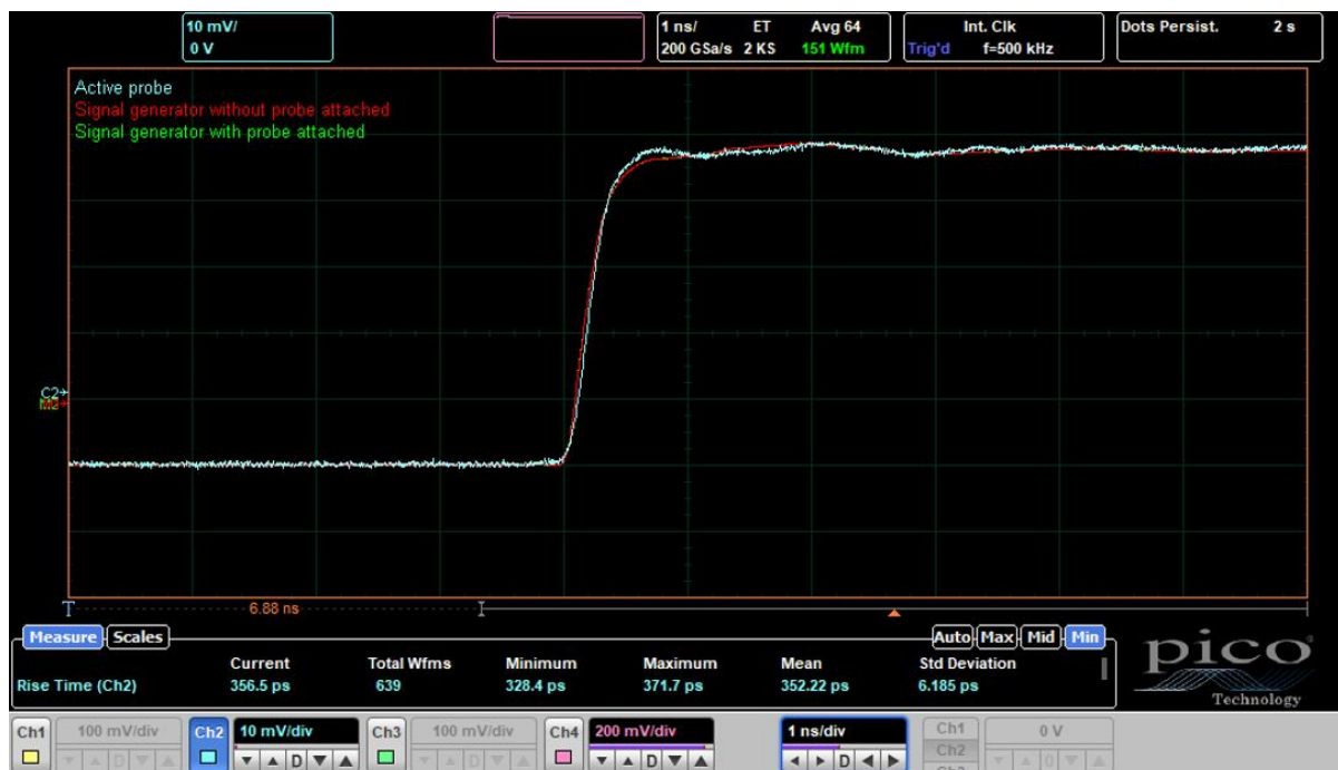
Figure 3. Typical probe step response to 350ps rising edge. Blue line is output from probe, sensing signal via exposed coplanar waveguide. Red line is signal generator signal measured directly by oscilloscope without probe attached. Green line is signal generator signal measured directly by oscilloscope with probe attached. Good reproduction of original signal displayed, and signal generator signal is entirely unaffected as red trace completely overlaps green trace.
